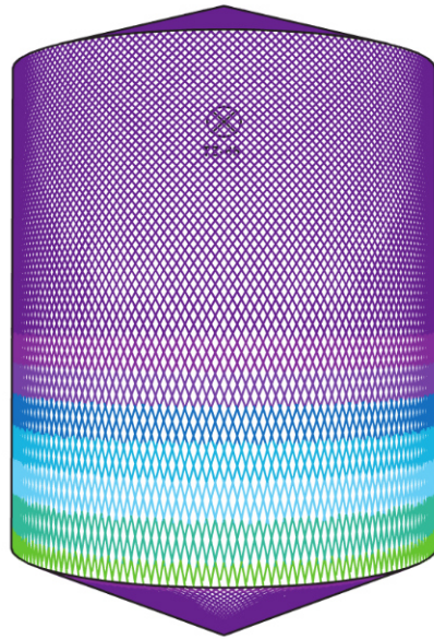
D8m H10m, Toftejorg TZ-66, 4 x ø10 mm, 0% Time = 23.3 min., Water consumption = 10868 l
